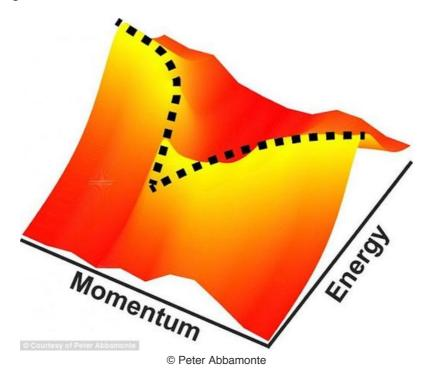
To uncover the elusive form of matter, the researchers developed a new technique called momentum-resolved electron energy-loss spectroscopy (M-EELS), which is more sensitive to excitations than other meths. The image shows the relationship between momentum and energy.
